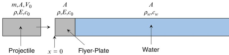
**Fig. 35.4** Schematic of the plate-impact and transmission-reflection problem at two interfaces – (1) projectile-flyer plate and (2) flyer-plate-water
